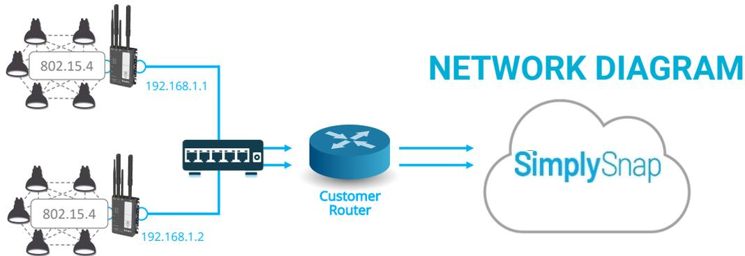
All communication with the internet is initiated through an outbound connection from the Synapse gateway. No inbound connections are initiated. The outbound ports required to facilitate network connectivity are listed below.
