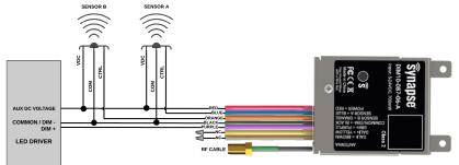
**DIM to OFF Wiring Diagram**
